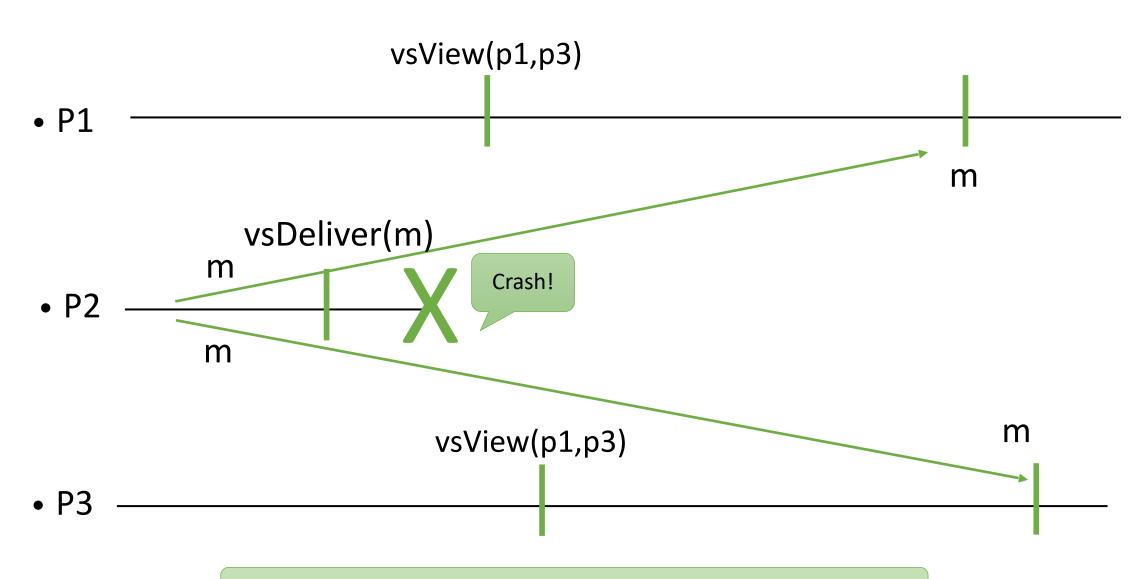
The message m is delivered in P2 but is not delivered in P1 and P3.
