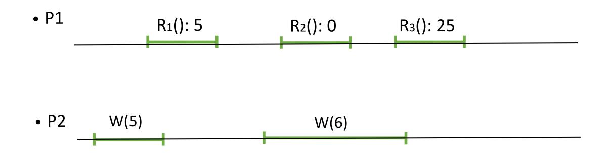
Just a so-called safe execution. Not a regular execution. Not an atomic execution. R2 does not return the value of a previous or concurrent write. No matter where W(6) is linearized, the return value of R2 cannot be justified.
